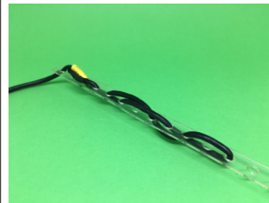
Example of how to adjust the wires over the plastic spacer
