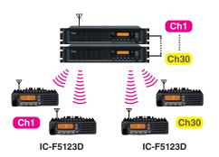
The IC-F5123D series can be used in an IDAS single-site trunking system.
