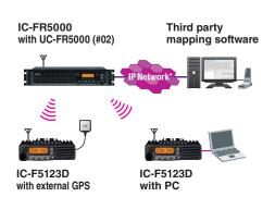
When used with an external GPS receiver, the IC-F5123D series can transmit accurate position data for use with vehicle management applications.
