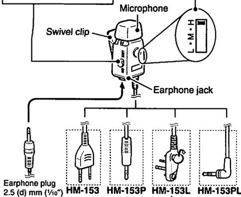
Insert the HM-153L, then tighten the screws of the plug.
