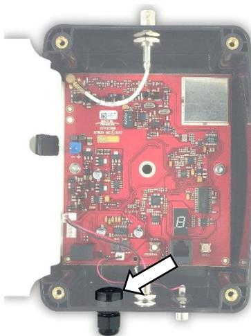
6. Install the Heyco strain relief included with cable assembly 60201127. Do not tighten the sealing nut at this time.
