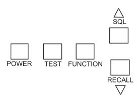
**POWER:** Press to turn on and off. Press and hold two seconds to activate backlight.
