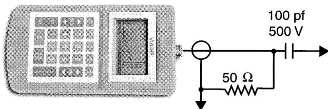
The VIA-HF is also suitable for calibration of receivers and signal peaking/alignment.
