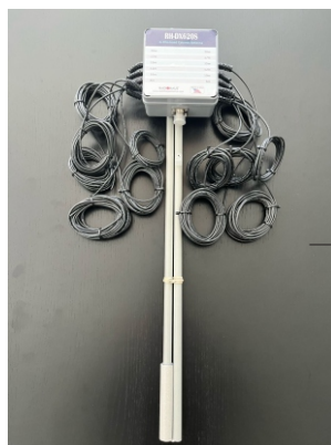
1 Foldable junction box arm with antenna elements
