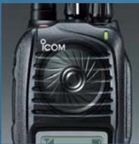
The built-in BTL amplifier doubles the audio output power and the large 40 mm speaker delivers loud 800 mW (typ.) audio to receive all calls under noisy environments.
